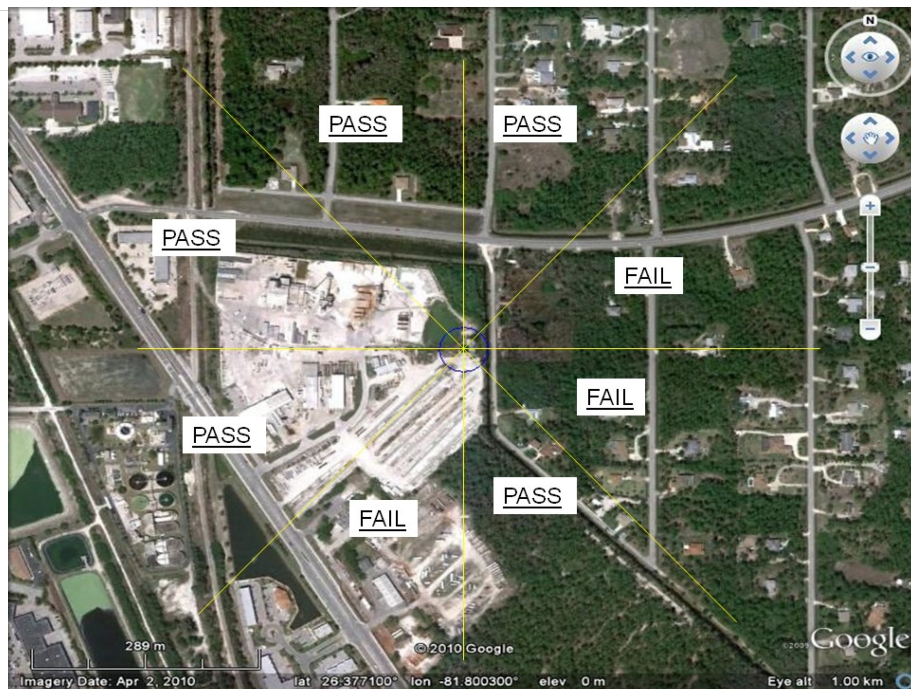
Fig 1. Example mesonet station, showing when wind observations from this site would be used (PASS) or not (FAIL) based on observed wind direction. The goal is to use wind observations when the flow is not obstructed, and to reject the observations when flow is obstructed.
